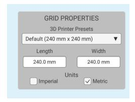
This allows the user to set the size of the workplane below the model. This can be used as a reference to see how large the model would be in real life.
